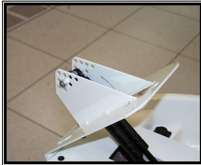
Figure 7.4.1 Pin Bolt on Upper Hinge Assembly.
