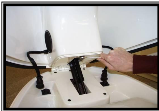
Figure 7.1.2 Removing Flange Bolt.
