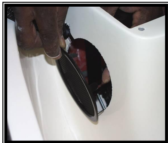
Figure 7.3.3 Removing Heater Intake Screens.
