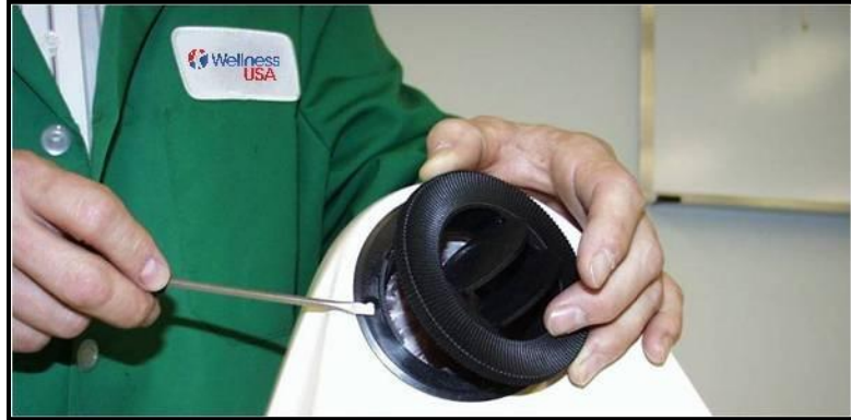
Figure 7.16.1 Removing Face Air Vent(s).
