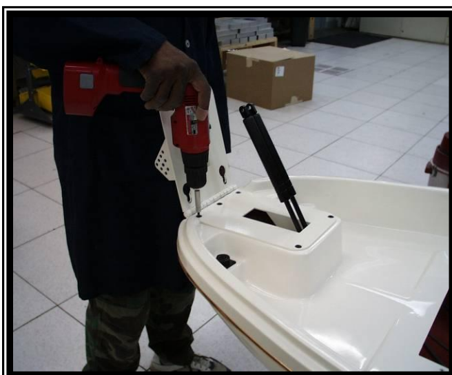
Figure 7.6.2 Removing Hinge Plate Screws on Base Chassis.
