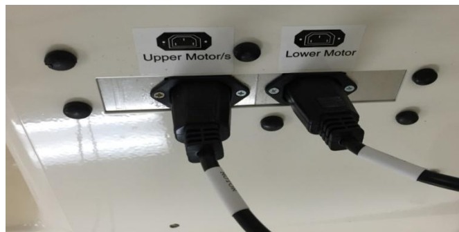
Figure 7.7.3 Disconnect Electrical Cords from Electrical Panel Cover.
