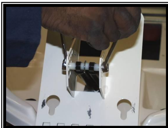
Figure 7.6.1 Removing Strut Pin Bolt and Nylon Spacers on Upper Hinge Assembly.
