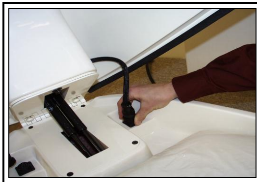
Figure 7.1.1 Releasing Electrical Connectors.
