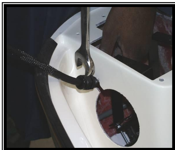
Figure 7.3.4 Removing Heater Harness.
